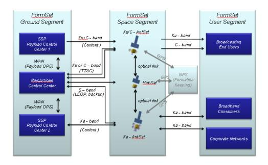
**Space Segment** FormSat space segment is composed of reception and transmission bent-pipe satellites, AntSat, and processing satellite, HubSat, rotating in a 24 hours ellipse in geosynchronous orbit.
