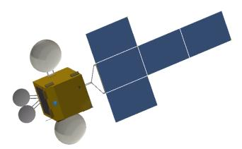
The Ka-AntSat's are better suited for the provision of corporate network and consumer broadband services with multibeam coverage of 0.75 deg half-power bandwidth. On-board processing and therefore single hop end-to-end communication is provided by the HubSat in orbit. CONUS coverage is provided with 48 beams leading to a capacity of 4 Gbps. FormSat scalability allows reaching a maximum system capacity of 30 Gbps.
