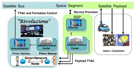
The satellite service provider ground segment deals with all issues that are related to the provision of the service. The payload control center (PCC) is in charge of the planning of the payload operations (payload configuration, processing capacity, ISL bandwidth), which is provided to the SCC as the central entity that coordinates the sharing of on-board resources. The satellite service provider uploads the service content to the satellites via the Gateway Earth Station (GES).
