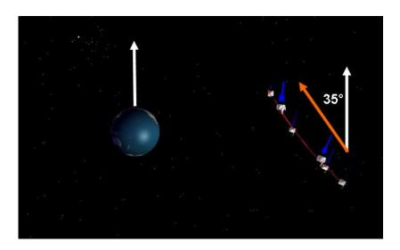
The satellites are equipped with a GPS device for absolute navigation. For autonomous control, the absolute positions are distributed via inter-satellite links, allowing safe formation flight without need for ground control. In case of contingency, the system can also be operated via a conventional TT&C link.
